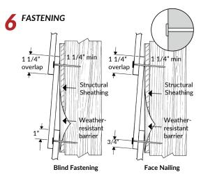
Fasteners must penetrate a minimum of 1-1/4" into structural framing.
